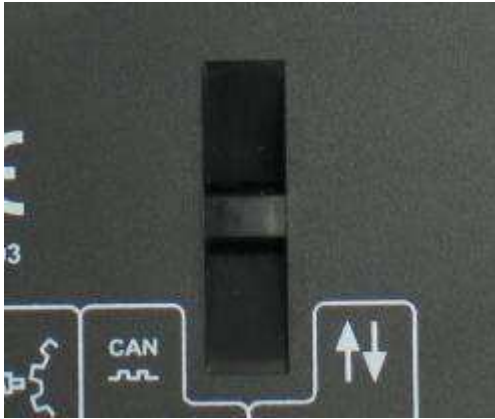
Cable tie fixing point
